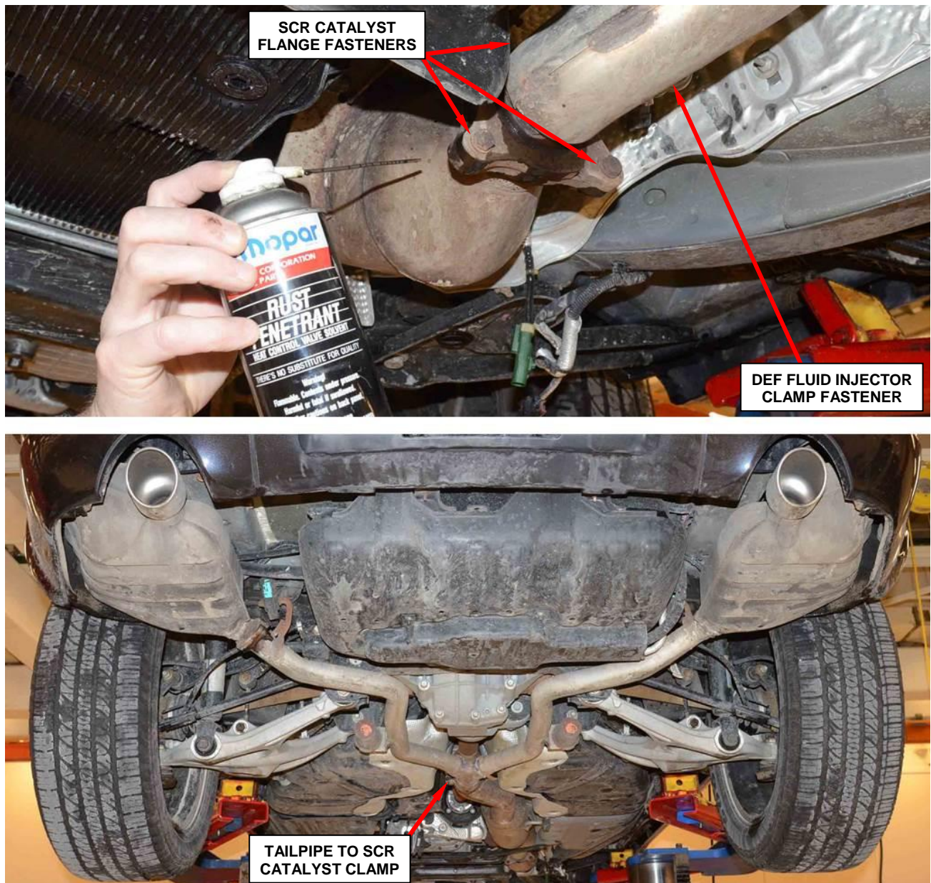
Figure 3 – Saturate Exhaust Fasteners with Penetrating Lubricant
